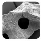
The macroporous structure enables migration of cells, penetration of blood vessels and integration of the particles
