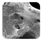
The capillary effect of the micropores leads to a quick blood uptake of the material
