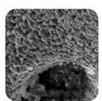
The rough surface ensures an excellent and homogenous adhesion of cells and proteins
